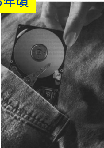
Figure 18-18 The IBM Travelstar 5 GT has the equivalent capacity of all the 350 disk files produced, and it is small enough to fit in a shirt pocket. [courtesy of IBM Corporation.]
